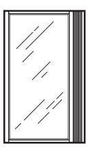
**General:** Furnish and install as shown on plans, a STYLEMATE® Pivot Door as manufactured by E.L. Mustee & Sons, Inc. Model \_\_\_\_\_\_ shall be a pivot-style door with a bright (Bright Silver, Black Bronze) finish, aluminum frame and clear tempered safety glass panel. Continuous pull handle with magnetic seal. Out-of-plumb condition up to 1" can be adjusted at latch jamb. Can be installed for right or left opening. Shall meet ANSI Specifications Z97.1
