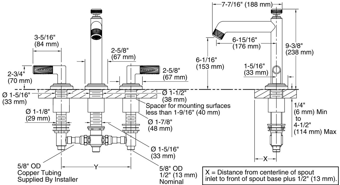
X = Distance from centerline of spout inlet to front of spout base plus 1/2" (13 mm).
