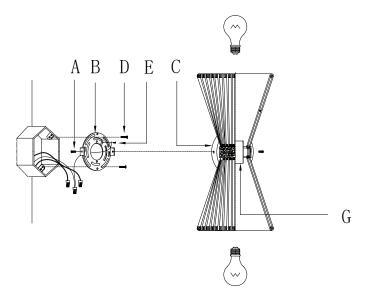
Note: If the shade needs to be removed for any reason. Use a long screwdriver through the shade to turn the screw to remove the shade.
